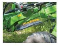
C) The fingerbar mower attachment with hydraulic boom is a versatile attachment for hedge cutting and trimming, mowing long hay etc. The hydraulic boom gives a 3500mm outreach and can be extended on both sides of the Avant loader with a cutting width of 1200mm. The strong fingerbar type cutting head can cut branches up to a maximum of 25mm.
